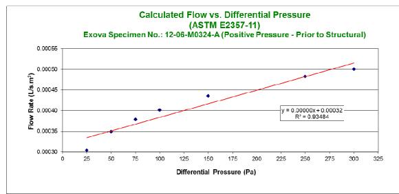
Figure 6 – Exova Specimen No.: 12-06-M0324-A Infiltration Air Leakage Prior to Structural Loading
