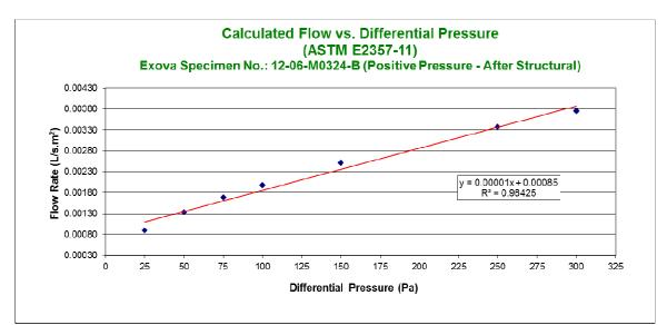
Figure 12 – Exova Specimen No.: 12-06-M0324-B Infiltration Air Leakage After Structural Loading
