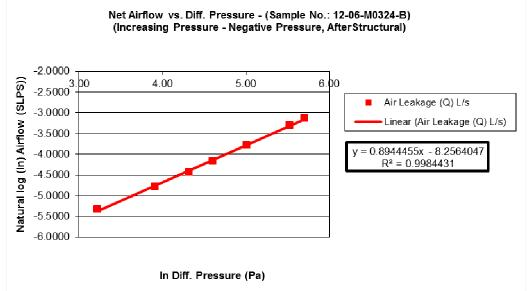
Figure C-3 – Exova Specimen 12-06-M0324-B Exfiltration Log/Log Graph After Structural Cycling
