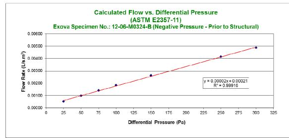
Figure 9 – Exova Specimen No.: 12-06-M0324-B Exfiltration Air Leakage Prior to Structural Loading
