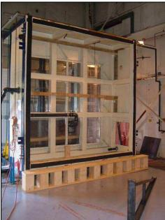
Figure 1 – Testing Chamber Prior to Specimen Installation Displaying Location of Air Seal (Stock Photo)
