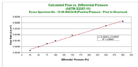
Figure 11 – Exova Specimen No.: 12-06-M0324-B Infiltration Air Leakage Prior to Structural Loading
