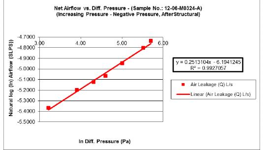
Figure B-3 – Exova Specimen 12-06-M0324-A Exfiltration Log/Log Graph After Structural Cycling
