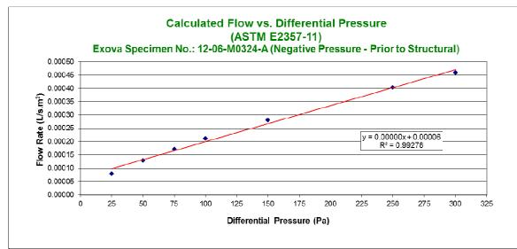
Figure 4 – Exova Specimen No.: 12-06-M0324-A Exfiltration Air Leakage Prior to Structural Loading
