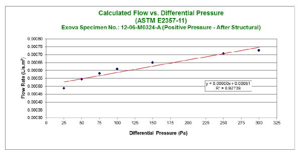
Figure 7 – Exova Specimen No.: 12-06-M0324-A Infiltration Air Leakage After Structural Loading
