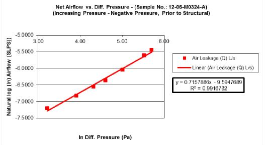
Figure B-1 – Exova Specimen 12-06-M0324-A Exfiltration Log/Log Graph Prior to Structural Cycling
