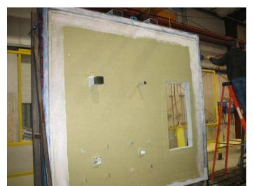
Figure E-9 – Application of LATICRETE Transition Tape Primer around Perimeter Wall / Specimen Transporter Frame Interface
