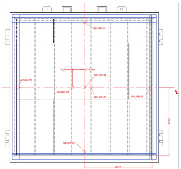
Figure 8 – Exova Specimen 12-06-M0324-A Gauge Locations
