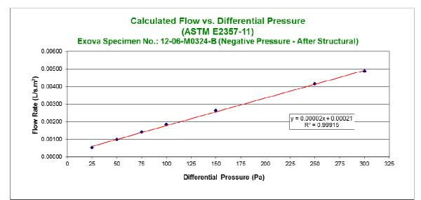
Figure 10 – Exova Specimen No.: 12-06-M0324-B Exfiltration Air Leakage After Structural Loading
