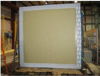
Figure D-2 – Completed Air Barrier Installation (Sheathing Joints Sealed, Second Coat of LATICRETE Air & Water Barrier Applied and LATICRETE Transition Tape and LATICRETE Flexible Sealing Tape Applied)
