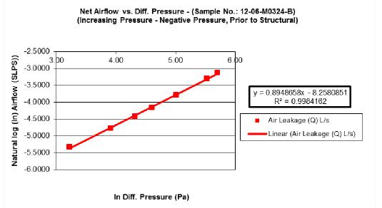
Figure C-1 – Exova Specimen 12-06-M0324-B Exfiltration Log/Log Graph Prior to Structural Cycling
