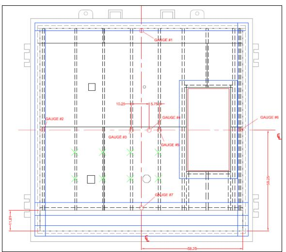
Figure 13 – Exova Specimen 12-06-M0324-B Gauge and Penetration Locations
