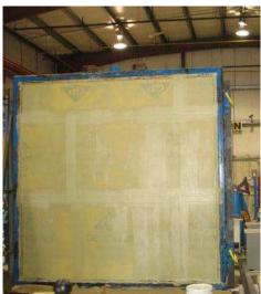
Figure D-1 – Sheathed Opaque Wall Section (Sheathing Joints Sealed and First Coat of LATICRETE Air & Water Barrier Applied)
