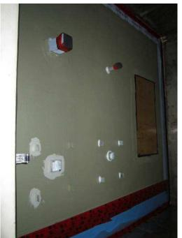
Figure E-13 – Completed Wall Assembly (red Tuck Tape along Foundation Interface used for Extraneous Bagging Purposes)
