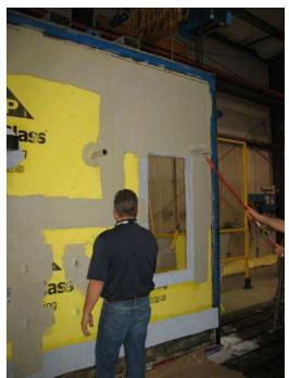
Figure E-6 – Application of LATICRETE Air & Water Barrier
