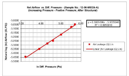
Figure B-4 – Exova Specimen 12-06-M0324-A Infiltration Log/Log Graph After Structural Cycling
