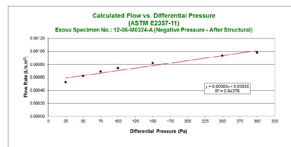
Figure 5 – Exova Specimen No.: 12-06-M0324-A Exfiltration Air Leakage After Structural Loading
